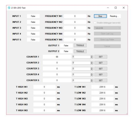
The test configuration will acquire the measure from the Modbus registers, you can also command the outputs and set counters to a value.
