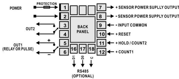
Figure 6 – Electrical connections of NC400-6
